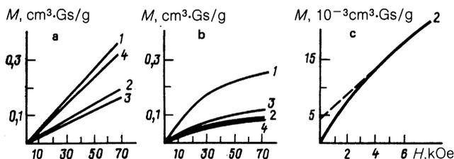
FIG. 3. Magnetization of the  $\text{CuGeO}_3$  crystal for three crystallographic axes at different temperatures: a— $T = 8$  K; b— $T = 2$  K; c— $T = 4$  K. Curves 1, 2, and 3 correspond to the magnetic field parallel to the a, b, and c crystal axes, respectively; curve 4 is calculated by the Monte Carlo method for temperatures above and below the Néel temperature ( $T_N = 7$  K). The dashed curve in part c shows the spontaneous magnetic moment  $M$  along the b crystal axis.
