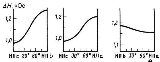
FIG. 8. Angular dependence of the EPR line width of the  $\text{CuGeO}_3$  crystal.
