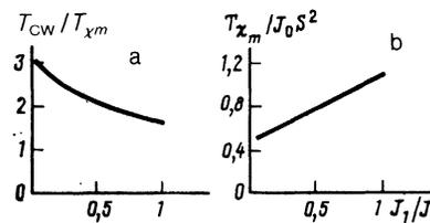
FIG. 10. Variation of  $T_{CW}/T_{\chi_m}$  and of  $T_{\chi_m}/J_0 S^2$  with  $J_1/J_0$ , calculated by the Monte Carlo method.
