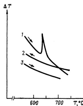
FIG. 1. Thermograms of amorphous and crystalline  $\text{CuGeO}_3$ : 1—amorphous sample heated at a rate of 4.5 deg/min; 2—amorphous sample cooled after heating to 950 °C; 3—crystalline sample heated at a rate of 4.5 deg/min.
