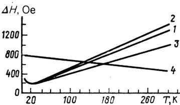
FIG. 6. Variation of the EPR line width with temperature for crystalline and amorphous  $\text{CuGeO}_3$ : 1— $\mathbf{H} \parallel \mathbf{a}$ ; 2— $\mathbf{H} \parallel \mathbf{b}$ ; 3— $\mathbf{H} \parallel \mathbf{c}$ ; 4—amorphous sample.
