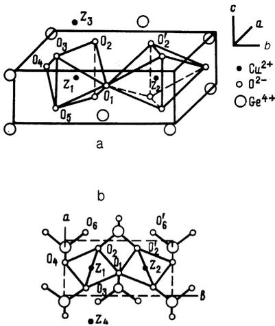
FIG. 2. Crystal structure of  $\text{CuGeO}_3$  (not all Ge atoms are shown in part a).
