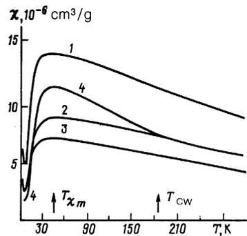
FIG. 4. Susceptibility of the  $\text{CuGeO}_3$  crystal for three crystallographic axes. Curves 1, 2, and 3 correspond to the susceptibility along the a, b, and c crystal axes, respectively; curve 4 is calculated by the Monte Carlo method. The temperature of maximum of susceptibility,  $T_{\chi m}$ , and the temperature  $T_{cW}$ , where the susceptibility departs from the Curie-Weiss law, are shown by arrows.
