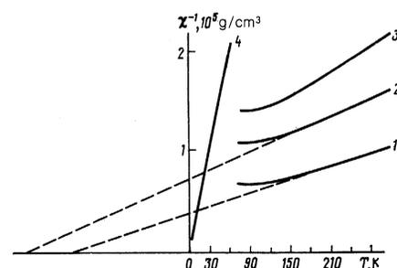
FIG. 5. Dependence of the inverse susceptibility on temperature for crystalline  $\text{CuGeO}_3$ . Curve notation is the same as in Fig. 4. Curve 4 shows the dependence of the inverse susceptibility on temperature for amorphous  $\text{CuGeO}_3$ .
