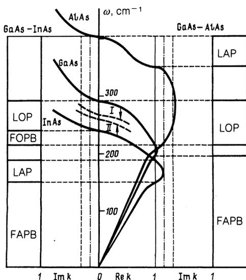
FIG. 1. Dispersion relations for the bulk materials AlAs, GaAs and InAs in the regions of real and imaginary values of the wave vectors. The vertical dashed and dashed-dot lines denote values of  $(\text{Im } k)^{-1}$  corresponding to attenuation of the vibrations in, respectively, one and two monolayers.
