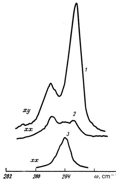
FIG. 4. Spectra of the SL  $(\text{GaAs})_6(\text{InAs})_2$  at  $T = 10$  K in the optical frequency region (1, 2— $\lambda_i = 488$  nm, 3— $\lambda_i = 652.8$  nm).
