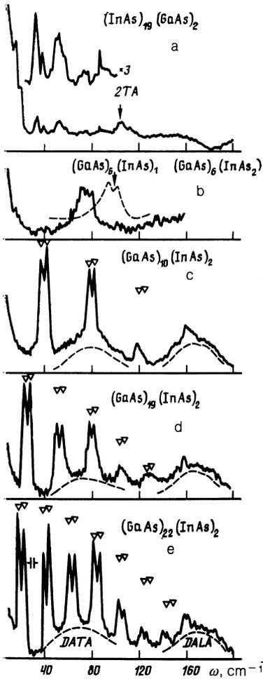
FIG. 3. RS spectra ( $T = 295$  K) in the acoustic frequency region for (a) type II SL's and (b, c, d, e) type I SL's.
