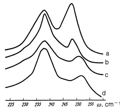
FIG. 10. RS spectra of a) solutions  $\text{In}_x\text{Ga}_{1-x}\text{As}$  for  $x = 0.95$  and the SL's b)  $(\text{InAs})_{10}(\text{GaAs})_{0.5}$ , c)  $(\text{InAs})_{10}(\text{GaAs})_1$ , d)  $(\text{InAs})_{10}(\text{GaAs})_2$  in  $xy$  geometry at  $T = 295$  K.
