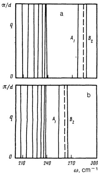
FIG. 9. Theoretical dispersion relation for the SL  $(\text{InAs})_{10}(\text{GaAs})$  a) without taking account of mechanical stresses in a GaAs layer and b) taking account of a deformation  $\xi \sim 7\%$  in a GaAs layer. The dashed lines indicate the solutions obtained for the SL  $(\text{InAs})_{10}(\text{GaAs})_1$ .
