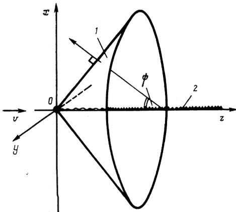
FIG. 2. Geometry of the problem. The analysis is carried out in the rest frame of the particle, which is moving at a velocity  $-v$ . The particle is at the origin. Surface 1 is the Mach cone; the heated jet (2) forms at the axis.
