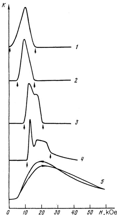
FIG. 1. Plots of EMAT efficiency  $K(H)$  vs the external magnetic field at  $\mathbf{H} \parallel \mathbf{a}$ : 1— $T = 82$  K, attenuation 0 dB; 2—119 K, 5 dB; 3—141 K, 15 dB; 4—172 K, 21 dB; 5—181 K, 12 dB. The arrows show the fields of the start and end, designated in the text by  $H_1$  and  $H_2$ , respectively, of the effective ultrasound excitation.
