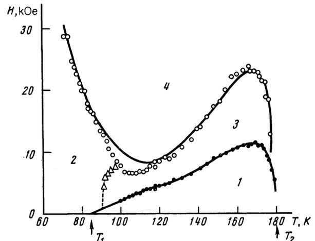
FIG. 6. The same for  $\mathbf{H} \parallel \mathbf{b}$ : 2—angle phase, upper line—calculated from Eq. (18),  $\Delta$ —experimental points separating the region with  $K(H)$  hysteresis from the region without hysteresis.
