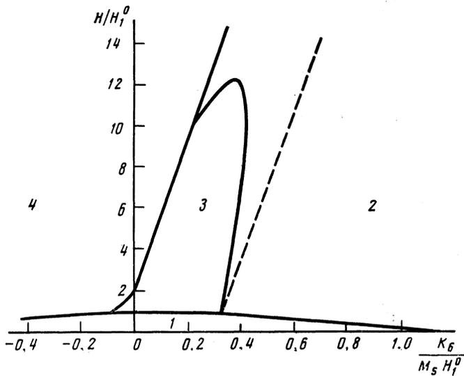
FIG. 4. Calculation of the phase diagram of Dy for  $\psi = 30^\circ$  ( $\mathbf{H} \parallel \mathbf{a}$ ) at  $K_6 < 0$  and for  $\psi = (2/3)^\circ$  at  $K_6 > 0.1$ —helicoid, 2—angle phase; 3—fan phase; 4—collinear phase. Dashed—boundary between fan-fold and canted phase at  $\psi = 0^\circ$  ( $\mathbf{H} \parallel \mathbf{b}$ ).
