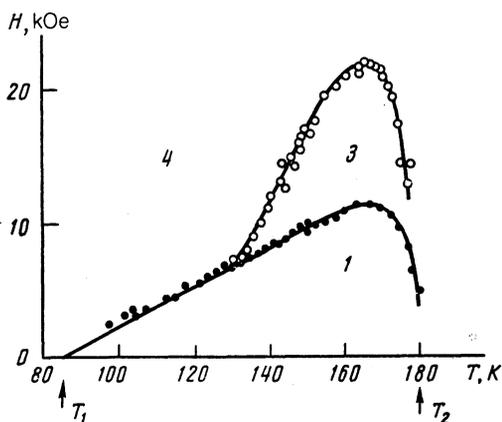
FIG. 5. Phase diagram of Dy for  $\mathbf{H} \parallel \mathbf{a}$ : 1—helicoid, 3—fan phase, 4—collinear phase,  $H$ —internal magnetic field. Experimental points:  $\bullet$ —field  $H_1$ ,  $\circ$ —field  $H_2$ .
