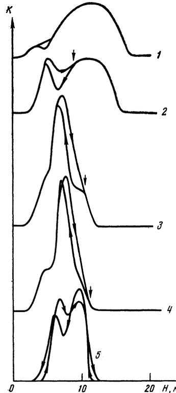
FIG. 3. Plots of  $K(H)$  at  $\mathbf{H} \parallel \mathbf{b}$ : 1— $T = 91$  K; 2— $92$  K; 3— $98.5$  K; 4— $101$  K; 5— $119$  K the arrows mark the fields at which the hysteresis processes terminate.
