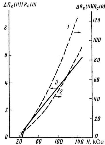
FIG. 12. Dependence of the magnetoresistance  $\Delta R_c(H)/R_c(0)$  on the field lying in the  $ab$  plane: 1)  $\mathbf{H} \perp (\mathbf{a} + \mathbf{b})$ ; 2)  $\mathbf{H} \parallel \mathbf{a}$ ; 3)  $\mathbf{H} \perp \mathbf{a}$ .
