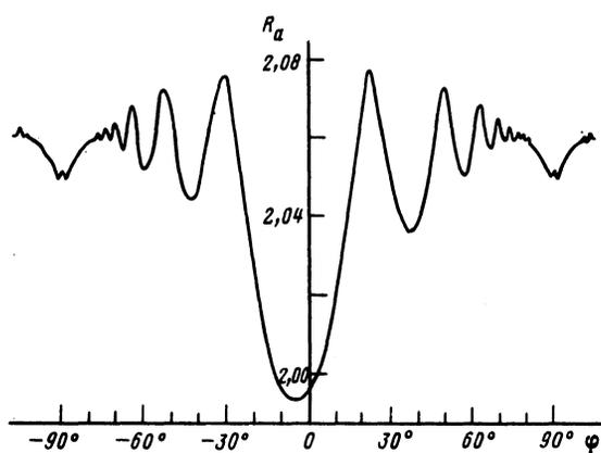
FIG. 2. Dependence of the resistance  $R_a$  ( $10^{-2} \Omega$ ) on the angle  $\varphi$  between the direction of the field in the  $b'c^*$  plane ( $H \perp a$ ) and the  $c^*$  axis;  $H = 150$  kOe,  $T = 1.45$  K.
