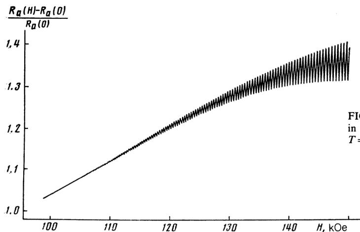
FIG. 7. Field dependence of the resistance  $R_d$  in the  $\mathbf{H} \perp \mathbf{b}'$  configuration in the region of the first local maximum shown in Fig. 1a ( $\varphi \approx 17^\circ$ );  $T = 1.45$  K.
