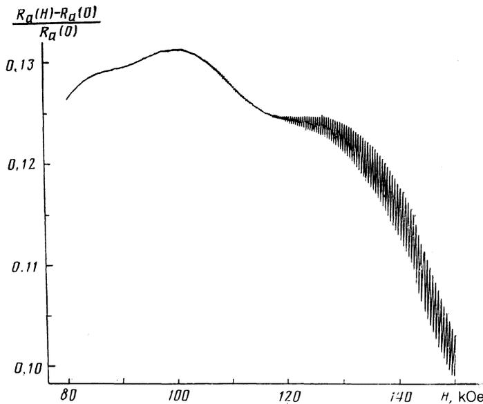
FIG. 5. Field dependence of the magnetoresistance along the  $a$  axis in the  $\mathbf{H} \perp \mathbf{b}'$  configuration;  $\varphi \approx -17^\circ$ ,  $T = 1.45$  K.
