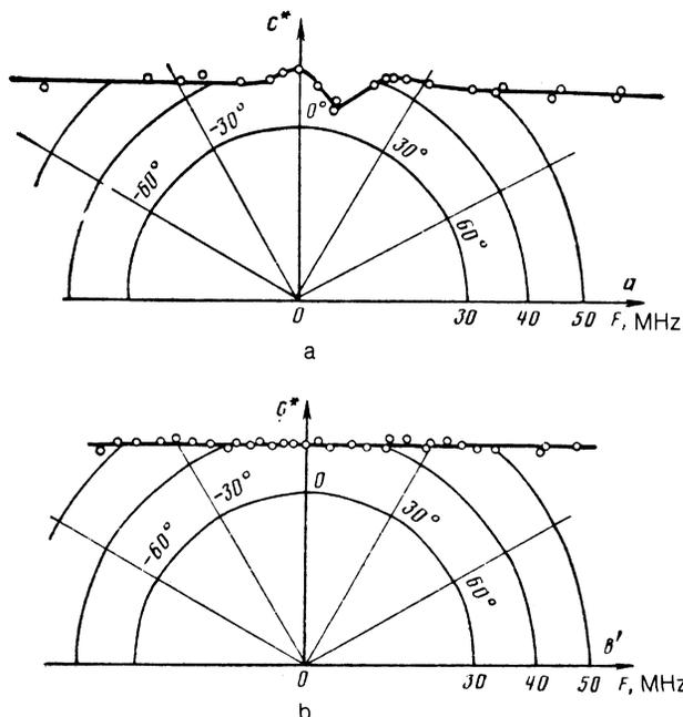
FIG. 9. Dependence of the frequency of fast Shubnikov-de Haas oscillations on the angle between the field and the  $c^*$  axis, plotted in polar coordinates; (a)  $\mathbf{H} \perp \mathbf{b}'$ ; b)  $\mathbf{H} \perp \mathbf{a}$ .
