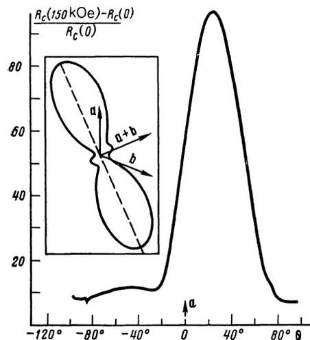
FIG. 4. Dependence of the transverse magnetoresistance  $R_c$  on the angle  $\theta$  between the direction of the field in the  $ab$  plane ( $H \perp c^*$ ) and the  $a$  axis;  $H = 150$  kOe,  $T = 1.45$  K. The inset shows the same dependence, but plotted using polar coordinates and indicating the directions of the crystallographic axes.
