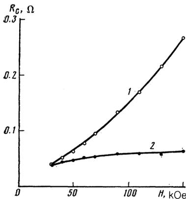
FIG. 11. Field dependence of the resistance  $R_c$  obtained in the  $\mathbf{H} \perp \mathbf{b}'$  configuration at the point of the first local maximum ( $\varphi \approx 17^\circ$ ). Curve 1 represents the total resistance and curve 2 is obtained by subtracting the absolute value of the peak of the dependence  $R(\varphi)$ .
