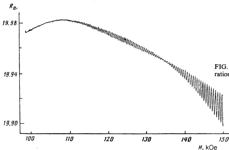
FIG. 6. Field dependence of the resistance  $R_a$  (m $\Omega$ ) in the  $\mathbf{H} \perp \mathbf{a}$  configuration;  $\varphi \approx -11^\circ$ ,  $T = 1.45$  K.
