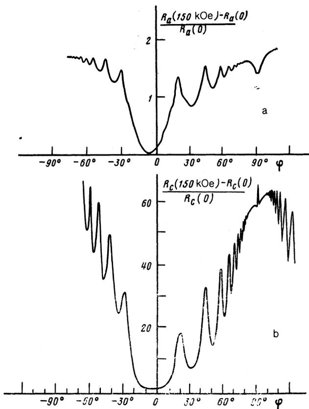
FIG. 1. Dependence of the magnetoresistance on the angle  $\varphi$  between the direction of the field in the  $ac^*$  plane ( $H \perp b'$ ) and the  $c^*$  axis;  $H = 150$  kOe,  $T = 1.45$  K. a) Resistance  $R_a$  along the  $a$  axis; b) resistance  $R_c$  across the  $ab$  plane.
