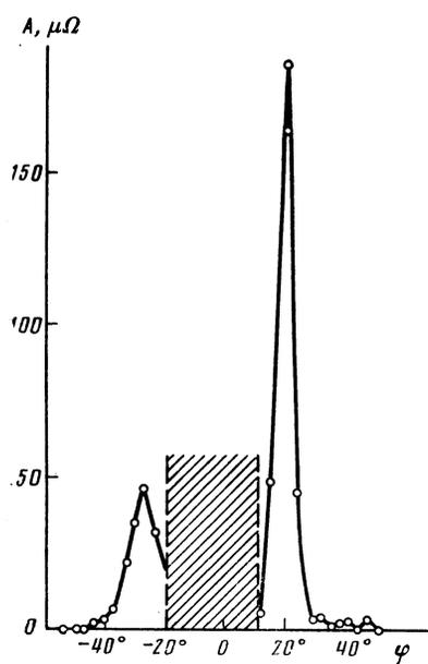
FIG. 8. Amplitude of the Shubnikov de Haas oscillations obtained in a field lying in the  $b'c^*$  plane;  $H = 150$  kOe,  $T = 1.45$  K. The shaded region is where significant beats occur.
