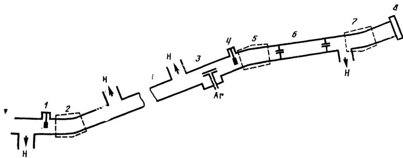
FIG. 1. Experimental layout. 1,4—Solid charge-exchange targets; 3—flowing gas target; 2,5,7—magnetic analyzers; 6—collision chamber; 8—system of proportional counters;  $H$ —diffusion pumps.
