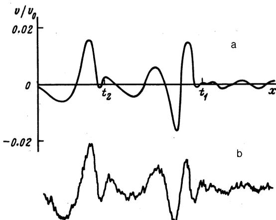
FIG. 3. Two-pulse free induction  $\sigma/\omega_1 = 0.5$ ,  $\omega_1/\delta = 0.5$ ,  $\omega_1 t_1 = 2\omega_1 t_2 = 8\pi$ . a—Theoretical; b—experimental.
