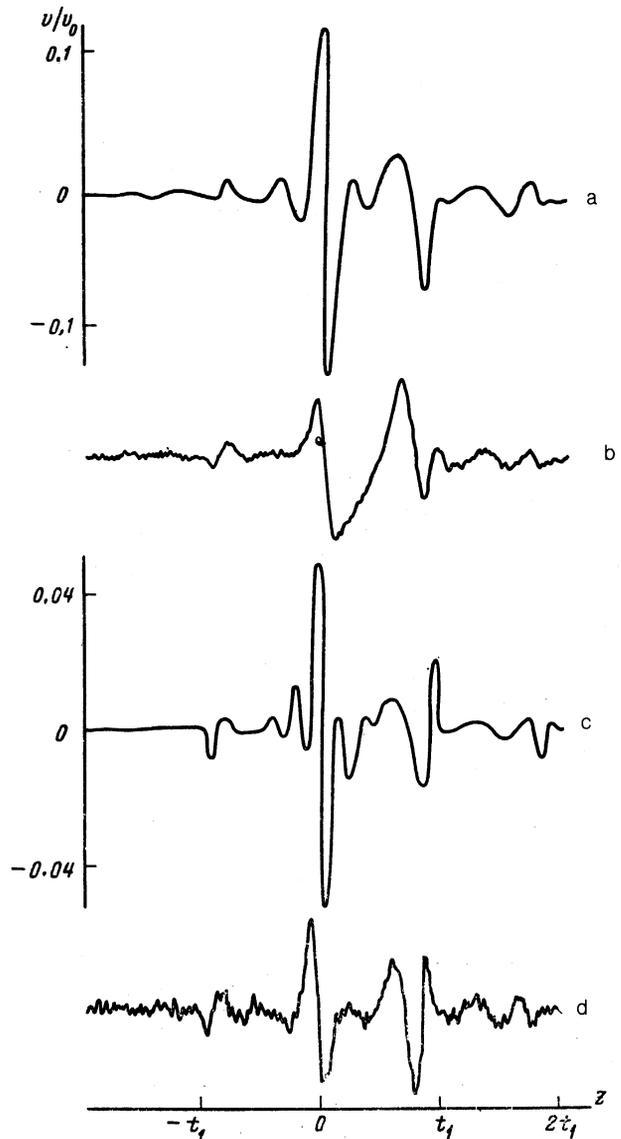
FIG. 4. Two-pulse echo for the case of equal pulse lengths  $\omega_1 t_1 = \omega_1 t_2 = 4\pi$ ,  $\tau = 5$  ms,  $t_1 = 1$  ms,  $\sigma/\omega_1 = 0.5$ ).  $\delta/\omega_1 = 1.5$ , a, c—Theoretical; b, d—experimental. a, b)  $\delta/\omega_1 = 1.5$ ; c, d) 2.5. The gain for oscilloscope trace d is twice that for case b.
