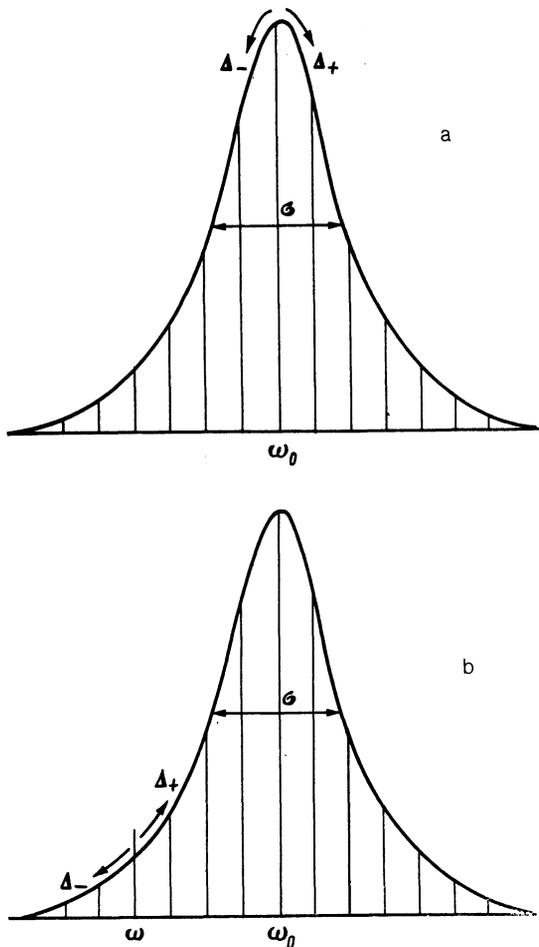
FIG. 2. Behavior of stationary points during (a) resonant and (b) nonresonant excitation of an inhomogeneous line.
