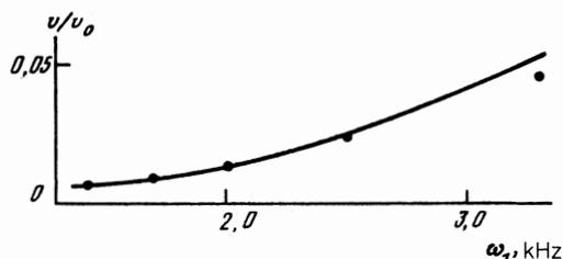
FIG. 5. Amplitude of the one-pulse echo versus the frequency of the rf field,  $\omega_1$ , for  $\omega_1 t_i = 20\pi$ ,  $\sigma = 2.6$  kHz, and  $\delta = 3.0$  kHz.
