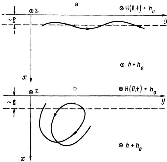
FIG. 1. The trajectories of the effective electrons in nonuniform magnetic fields (a) alternating in direction and (b) pointing in one direction only.
