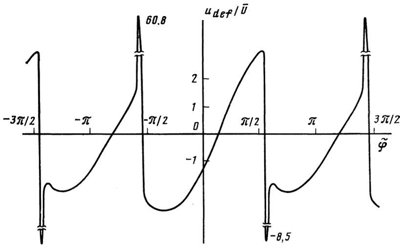
FIG. 2. The results of the calculation of the displacement  $u_{\text{def}}(\tilde{\varphi})$  ( $\tilde{\varphi} = \omega t - qk$ ) for values of the nonlinearity parameter  $b = 5$ , the external field  $h_0/2\mathcal{H} = 0.2$ , and  $\bar{\kappa} > 0$ .
