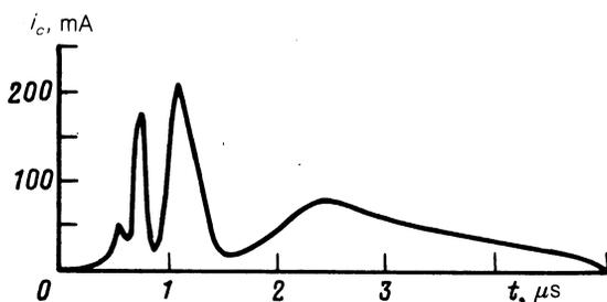
FIG. 7. Oscillograms of the ion current to the collectors.  $B = 0.2$  T,  $L = 6.5$  cm,  $\Phi \sim 3 \times 10^{10}$  W/cm<sup>2</sup>,  $\varphi = -3^\circ$ .
