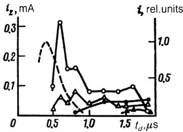
FIG. 9. Charge spectrum of carbon ions represented by  $i_z(t)$  for  $z = 1$  ( $\blacktriangle$ ),  $z = 2$  ( $\bullet$ ),  $z = 3$  ( $\triangle$ ), and  $z = 4$  ( $\circ$ ).  $B = 0.2$  T,  $L = 5$  cm,  $\Phi \sim 10^9$  W/cm $^2$ ,  $\varphi = +3^\circ$ , and amplitude of high-voltage pulses  $-3.9$  kV.
