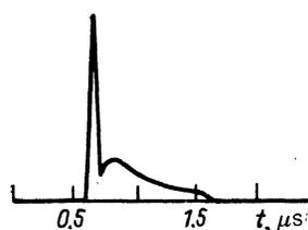
FIG. 1. Oscillogram of a CO<sub>2</sub> radiation pulse.
