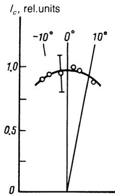
FIG. 4. Ion current reaching the collectors from the head part of a plasma in the region characterized by  $\beta \sim 1$ . The results were obtained for a carbon target;  $B = 0.2$  T,  $\Phi \sim 3 \times 10^{10}$  W/cm<sup>2</sup>,  $L = 5$  cm.
