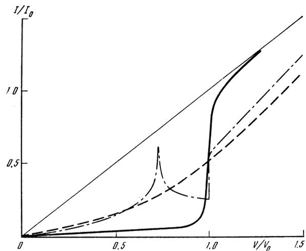
FIG. 3. Comparison of an experimental  $I(V)$  curve (bold solid curve) with a simple one-particle model [formula (1), dashed curve] and a model accounting for the proximity effect (dot and dash curve, see below, section 3). Here we have  $I_0 = V_0/R$ ,  $eV_0 = \Delta_{\text{BCS}}(T)$  for the experimental curve and model (1),  $eV_0 = \Delta_{\text{BCS}}(T) + \Omega$  for the model taking account of the proximity effect,  $t = 0.52$ .
