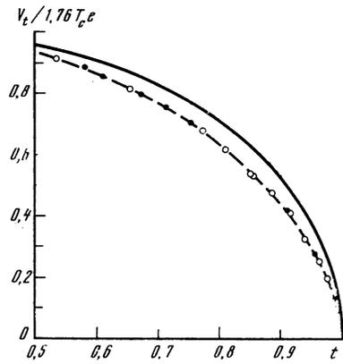
FIG. 2. Position of the inflection  $V_i$  on the  $I(V)$  curves plotted as a function of the reduced temperature  $t$ . The different designations on the points correspond to different contacts. The solid curve represents the width of the superconducting gap in BCS theory plotted as a function of the reduced temperature.
