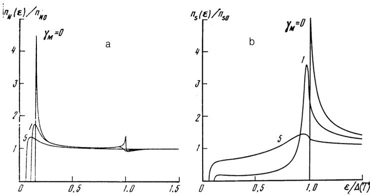
FIG. 5. State densities of the normal (a) and superconducting (b) banks of a contact for a number of parameters  $\gamma_M$  (indicated near the curves) for  $\gamma_B = 10$  ( $\eta_{N_0}, \eta_{S_0}$  are the normalized state densities of the banks).
