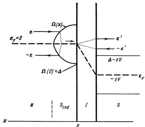
FIG. 6. Energy scheme of the proposed contact model.
