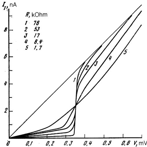
FIG. 4. Change in the shape of the  $I(V)$  curve of a contact upon successive applications of the point  $i = 1-5$  and a fixed temperature  $t = 0.52$ . Scale  $I_1$  corresponds to curve 1. We have  $I_i = I_1 R_1 / R_i$  for curves with  $i = 2-5$ .
