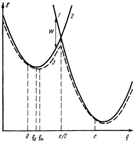
FIG. 2. The Coulomb energy  $E^{(n)}(q) - qV$  of quantum states with  $n = 0$  (curve 1) and  $n = 1$  (2) and the effective renormalized potential  $U(q)$  (3) versus the magnitude of the charge.
