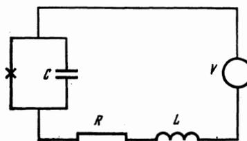
FIG. 1. Circuit connecting the tunnel junction to the external source.
