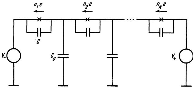
FIG. 4. Equivalent circuit of a chain of tunnel junctions.  $C$ —Self-capacitance of junction;  $C_0$ —capacitance between the electrodes of the junction and the substrate.
