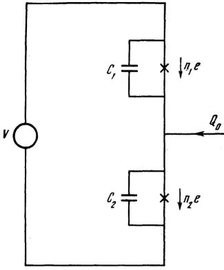
FIG. 3. Equivalent circuit of a one-electron tunnel transistor.
