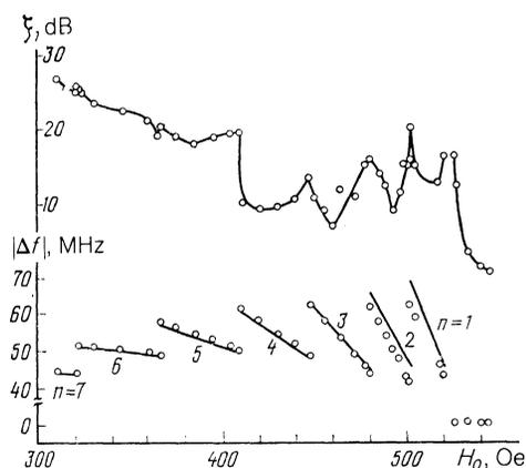
FIG. 3. Dependence of  $|\Delta f|$  (the deviation of the radiation frequency from half the pump frequency  $f_p/2$ ) and the supercriticality ratio  $\zeta$  at which this radiation appears on the value of the external magnetic field  $H_0$ . The solid traces in the lower part of the figure show the theoretical dependence of  $|\Delta f(H_0)|$  for nondegenerate excitation of RBMW with indices  $(n, n+1)$  for  $n = 1, 2, \dots, 7$ .
