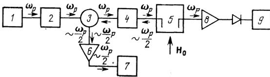
FIG. 2. Block diagram for the experimental setup: 1—pump oscillator with frequency 3.3 GHz; 2—gate; 3—wide-band circulator; 4—impedance transformer; 5—ferrite film with input and output antennas in a magnetic field; 6—amplifier at a frequency of  $1.65 \pm 0.25$  GHz; 7—spectrum analyzer; 8—amplifier at the pump frequency; 9—oscilloscope.
