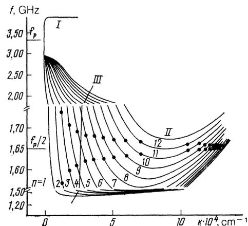
FIG. 1. Spectrum of waves of a tangentially magnetized YIG film of thickness  $16 \mu\text{m}$ ,  $H_i = 498 \text{ Oe}$ : I—SMW propagating perpendicular to  $H_i$ ; II—RBMW, propagating along  $H_i$ ; III—transverse elastic waves. For convenience, the part of the spectrum near half the value of the pump frequency is shown using an expanded scale. The numbers are the RBMW indices  $n$ , while the curves are the dispersion relations for the first twelve waves.
