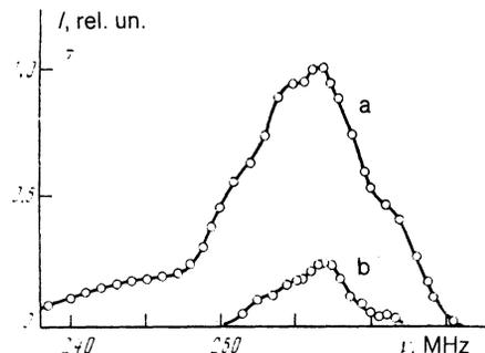
FIG. 3. Echo-signal amplitude  $I$  for sample with  $\delta = 0.17$  at  $T = 77 \text{ K}$  vs the excitation frequency  $\nu$  and the values  $n = 2$  (a) and 4 (b).
