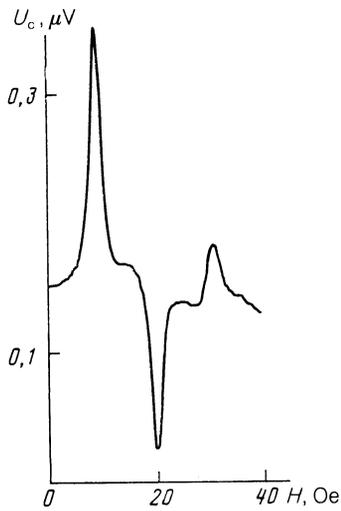
FIG. 4.  $U_c(H)$  at  $T = 1.7$  K with  $\mathbf{L} \parallel C_2$  and  $\mathbf{H} \perp \mathbf{L}$ .
