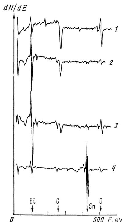
FIG. 1. Auger spectra of the surface of a bismuth sample. 1—Before the surface is cleaned by ion bombardment; 2—after the surface is cleaned by bombardment for 1 h by 150-eV  $Ar^+$  ions; 3—after the sample is heated at 420 K for 1 h; 4—after the deposition of the tin film. The sensitivity of the measurement apparatus was reduced by a factor of 2.5 for the recording of curve 4. The positions of characteristic Auger peaks along the energy scale are shown for bismuth, carbon, tin, and oxygen.
