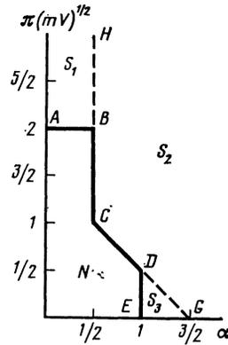
FIG. 5. Phase diagram of a chain of tunnel junctions with linear ohmic dissipation in the limit as  $MV \rightarrow \infty$ . With decrease of  $M$  the lines  $AB$  and  $CG$  shift upwards. The dashed lines are those of the additional phase transitions on which the exponent  $\lambda$  of the temperature dependence of the resistance has discontinuities.
