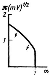
FIG. 2. Phase diagram of chain of tunnel junctions with linear ohmic dissipation (for  $M = 0$ ), obtained in Refs. 9 and 10 by a variational analysis. The arrows indicate the direction the displacement of the curved section of the interphase boundary with increase of  $M$ .
