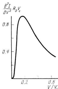
FIG. 3. Second derivative of the current with respect to voltage vs the voltage, for the case of a long tunnel junction.
