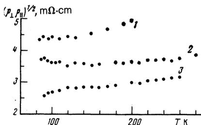
FIG. 2. Temperature dependence of  $(\rho_{\parallel}\rho_{\perp})^{1/2}$  for single crystals 1, 2, and 3 of Ref. 8.
