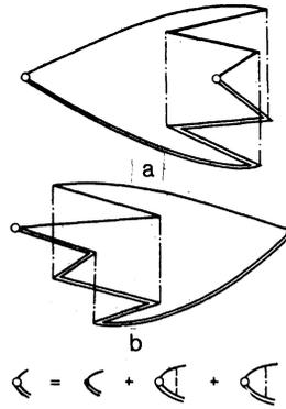
FIG. 1. Berezinskiĭ diagrams determining the quantum-mechanical correction to the conductivity in the case of a scattering by plane defects. Solid line—Retarded Green's functions; double line—advanced Green's function; dot-dashed line—line describing a scattering by plane defects; dashed line—impurity or phonon line, filled point—current vertex.
