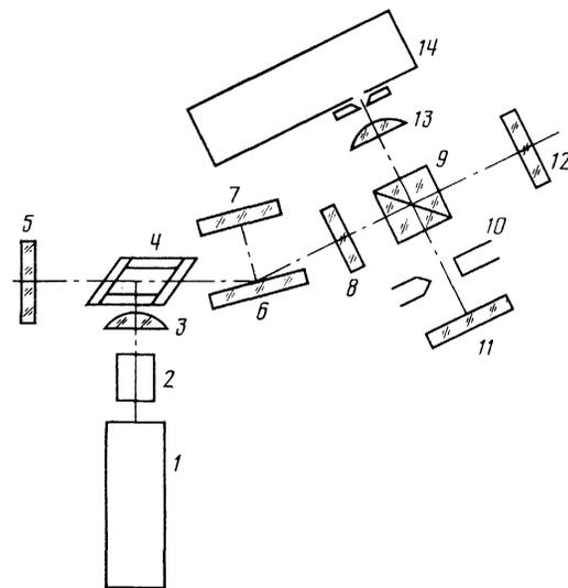
FIG. 2. Block diagram of apparatus: 1—ruby laser; 2—KDP crystal; 3, 13—cylindrical lenses; 4—cell containing the dye (rhodamine 6G or coumarin 153); 5—90% mirror; 6—diffraction grating; 7—100% mirror; 8—plane-parallel plate; 9—beam-splitting cube; 10—arc discharge (IBS-28); 11, 12—100% mirrors; 14—spectrograph.
