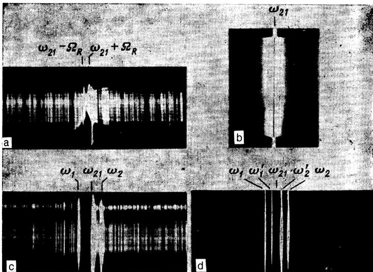
FIG. 5. Two-level system in a light field: a—amplification spectrum in the field of the monochromatic wave; b—generation spectrum in the field of the monochromatic pump; c, d—generation spectrum in the field of the biharmonic pump ( $\omega_1$  and  $\omega_2$ ) at frequencies  $\omega_{1,2} \pm \Delta\Omega/2$  and  $\omega_{1,2} \pm \Delta\Omega/3$ .
