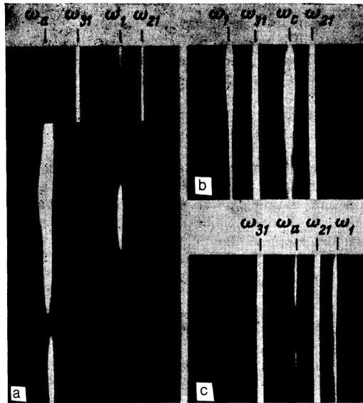
FIG. 6. Generation spectra for different detuning  $\omega_1 - \omega_2$  of the narrow-band line;  $\omega_{31}$  ( $\lambda = 589.0$  nm) and  $\omega_{21}$  ( $\lambda = 589.6$  nm)—reference lines produced by a sodium lamp;  $\omega_1$ —narrow-band pump radiation;  $\omega_c, \omega_a$ —generation lines that appear when sodium atoms are introduced into the cavity.
