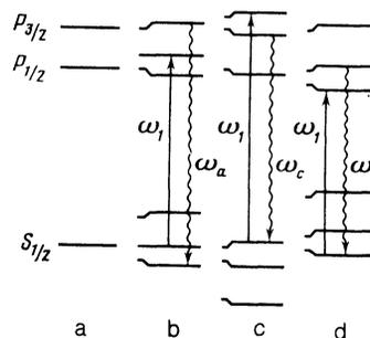
FIG. 7. Level scheme for sodium in the absence of the external field (a) and the quasilevel scheme produced by the narrow-band pump radiation  $\omega_1$  (b-d);  $\omega_a, \omega_c$ —transitions between quasilevels that correspond to the observed generation.
