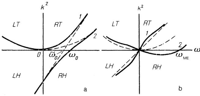
FIG. 1. Dispersion curves  $k_{1,2}^2 = k_{1,2}^2(\omega)$  near (a) and at (b) the transition point ( $\tilde{\omega}_0 \approx \omega_{ME}$  and  $\tilde{\omega}_0 = 0$ , respectively). The left- and right-polarized waves are labeled  $L$  and  $R$ , respectively;  $T, H$  stand for trigonometric and hyperbolic.
