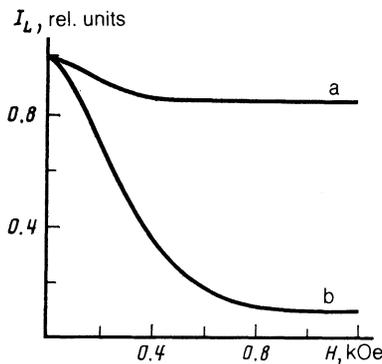
FIG. 1. Dependence of the integrated luminescence intensity  $I_L$  on the magnetic field applied to a sample of  $n$ -type InSb with an equilibrium carrier density  $n_0 = 8 \times 10^{13} \text{ cm}^{-3}$ : a)  $\mathbf{H} \perp \mathbf{k}$ ; b)  $\mathbf{H} \parallel \mathbf{k}$  ( $\mathbf{k}$  is the wave vector of the exciting radiation).
