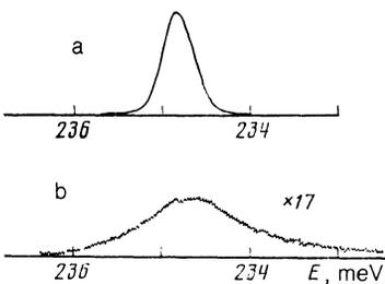
FIG. 2. Luminescence spectra of a sample of  $n$ -type InSb with an equilibrium carrier density  $n_0 = 8 \times 10^{13} \text{ cm}^{-3}$  in the absence (a) and presence (b) of a longitudinal magnetic field ( $H = 1 \text{ kOe}$ ).
