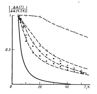
FIG. 5. Reduced temperature dependence of the magnetostriction in a 40kOe magnetic field. The dashed curves are calculated on the basis of Eq. (12). The notation is as follows: O)  $Tm_3Ga_5O_{12}$ ,  $H||[111]; \Delta$ )  $Dy_3Al_5O_{12}$ ,  $H||[111]; \Delta$ )  $Tb_3Al_5O_{12}$ ,  $H||[111]; \bullet$ )  $Yb_3Al_5O_{12}$ , H||[100]. The continuous curve represents a calculation based on Eq. (1) for  $Yb_3Al_5O_{12}$ .
