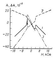
FIG. 6. Field dependence of the magnetostriction of  $Dy_3Al_5O_{12}$  at 1.35 K in H||[111]: 1) longitudinal magnetostriction; 2) transverse magnetostriction; 3) difference between the longitudinal and transverse magnetostrictions.
