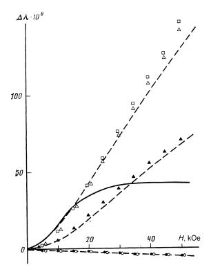
FIG. 4. Field dependence of the magnetostriction of  $Tb_3Al_5O_{12}$  at 4.2 K in the (110) and (100) planes. The notation is the same as in Fig. 2.
