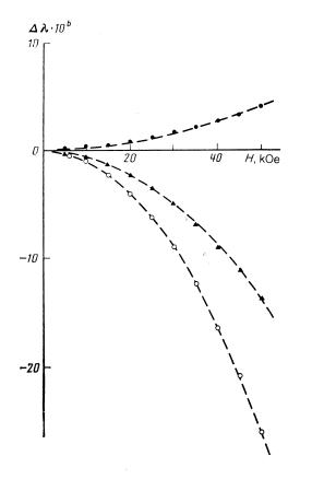
FIG. 1. Field dependence of the magnetostriction of  $Tm_3Ga_5O_{12}$  at 4.2 K in the (110) plane:  $\bigcirc$ ) H $\parallel$ [111];  $\blacktriangle$ ) H $\parallel$ [110];  $\bigoplus$ ) H $\parallel$ [001]. The dashed curves represent dependences calculated on the basis of Eq. (2).
