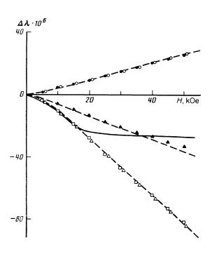
FIG. 3. Field dependence of the magnetostriction of  $Dy_3Al_5O_{12}$  at 4.2 K in the (110) and (100) planes. The notation is the same as in Fig. 2.
