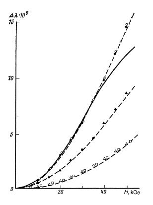
FIG. 2. Field dependence of the magnetostriction of  $Yb_3Al_3O_{12}$  at 4.2 K in the (110) plane:  $\Box$ )  $H \parallel [\bar{1}11], \land$ )  $H \parallel [\bar{1}10], \bullet$ )  $H \parallel [001]$  and the corresponding results for the (100) plane:  $\triangle$ )  $H \parallel [011]; \bigcirc$ )  $H \parallel [001]$ . The dashed curves are calculated using Eq. (12) when the continuous curves are based on Eq. (1).
