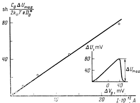
FIG. 3. Example of an analysis of the nonlinear characteristics in the case of filamentation of the Hall current. The inset shows the experimental dependence of the voltage between the drain and source on the gate voltage applied to sample No. 1.
