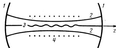
FIG. 3. Electron in an open resonator: 1) mirrors; 2) wave-beam caustic; 3) electron trajectory; 4) undulator.
