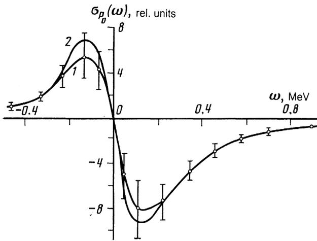
FIG. 3. Polarization-dependent part of the neutron-scattering cross section as a function of the energy transfer for  $\varphi = 22^\circ$ ,  $\theta = 4.5^\circ$ ,  $k\theta = 0.1 \text{ \AA}^{-1}$ , and  $\Delta T = T - T_c = 30^\circ$ : 1) fitting curve from Ref. 28; 2) function calculated using the expressions (22) and (26), (27).
