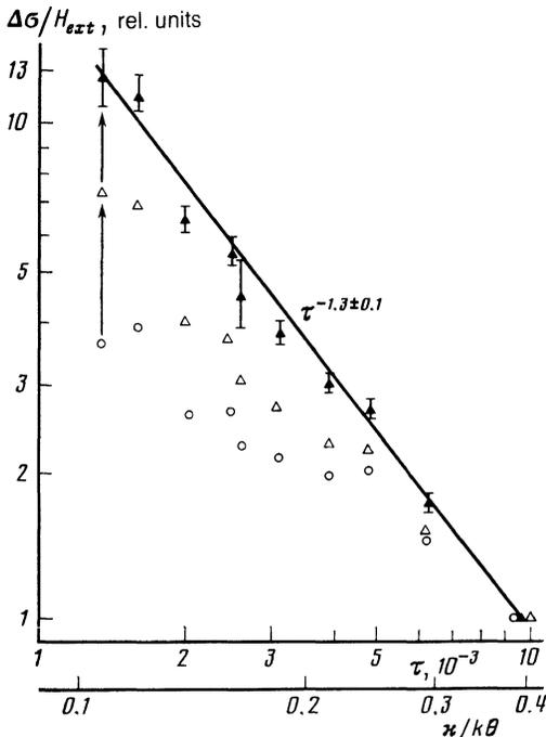
FIG. 4. Dependence of the scattering asymmetry  $\Delta\sigma$ , divided by  $H_{\text{ext}} = 22 \text{ Oe}$ , on  $\tau$  in the region  $k\theta > \kappa$  (the critical region):  $\circ$ —experimental data of Ref. 15,  $\triangle$ —the same data with allowance for the demagnetization in the scattering system;  $\blacktriangle$ —data with allowance for the demagnetization and the inelasticity of the scattering.
