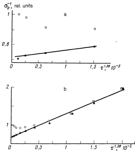
FIG. 2. Reciprocal of the polarization-independent part of the neutron-scattering cross section as a function of  $\kappa^2 \propto \tau^{1.38}$ :  $\circ$ —the experimental data of Ref. 15,  $\blacktriangle$ —the same data after allowance for the inelasticity of the scattering; a) the region  $\kappa > \xi$  (the critical region,  $\max(\kappa/k\theta) \cong 0.4$ ); b) the entire region of the measurements ( $\max(\kappa/k\theta) \cong 1.4$ ).
