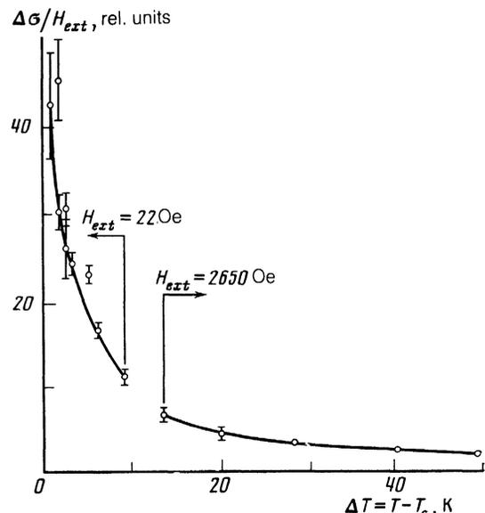
FIG. 5. Temperature dependence of the normalized scattering asymmetry for  $k\theta = 0.1 \text{ \AA}^{-1}$  and  $\varphi = 22^\circ$ . The solid line corresponds to the calculation based on the expression (29).
