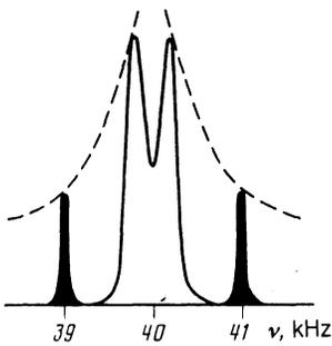
FIG. 3. Fourier spectra of collective oscillations of a system of parametric nuclear spin waves near the frequency  $\nu_{m1}/2 = 40$  kHz when  $\nu_{m2} = 39$  kHz (black peaks) and  $\nu_{m2} = 39.8$  kHz (white peak).
