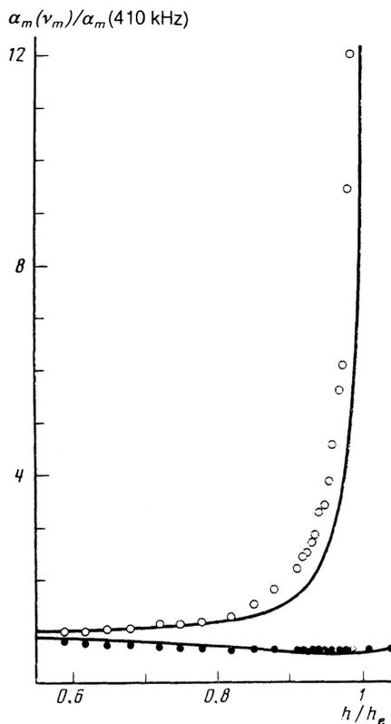
FIG. 2. Dependence of the reduced modulation response  $\alpha_m(\nu_m)/\alpha_m(410$  kHz) on the amplitude  $h$  of the microwave pump field for two typical frequencies: (○)  $\max \alpha_m(\nu_m)$  ( $\nu_m = 417.8$  kHz); (●)  $\min \alpha_m(\nu_m)$  ( $\nu_m = 419.5$  kHz). The continuous curves are calculated on the basis of Eq. (2) using the parameters given in the caption of Fig. 1.
