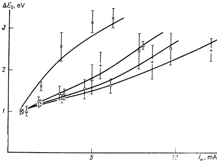
FIG. 9. Energy width  $\Delta E_0$  as a function of electron current in magnetic fields of strengths 4 (+), 3 (○), 2 (▲), and 1 (×) kG.
