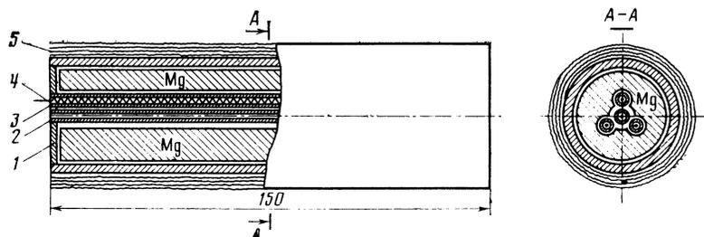
FIG. 3. Magnesium vapor target: 1—container with magnesium, 2—tube for passage of ion beam, 3—tubes for heaters, 4—heaters, 5—heat shield.
