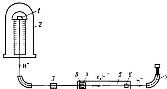
FIG. 2. Diagram of apparatus: 1—Source of  $H^-$  ions, 2—electrostatic accelerator, 3—magnesium vapor target, 4—electron gun, 5—solenoid, 6—electron collector, 7—spectrometer, 8—additional solenoid.
