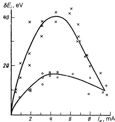
FIG. 7. Friction force as a function of electron current.  $B_0 = 3$  kG,  $\times - H^-$ ,  $\circ - H^+$ .
