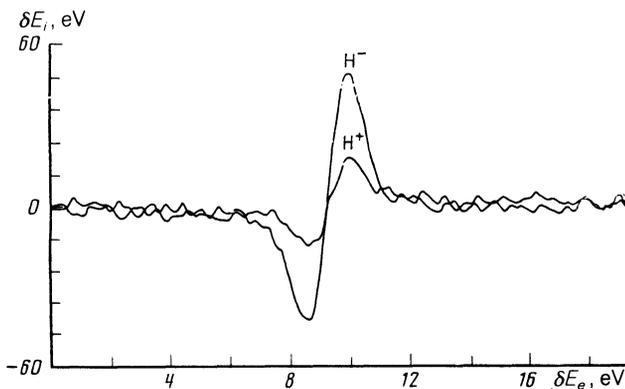
FIG. 6. Change of energy of ions of different signs as a function of electron energy for  $B_0 = 4$  kG and  $I_e = 3$  mA.
