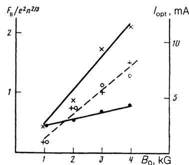
FIG. 8. Maximum friction force as a function of magnetic field strength (solid lines,  $\times - H^-$ ,  $\bullet - H^+$ ), expressed in units of  $e^2 n^{2/3}$ , and optimal electron beam current (dashed line,  $+ - H^-$ ,  $\bullet - H^+$ ).
