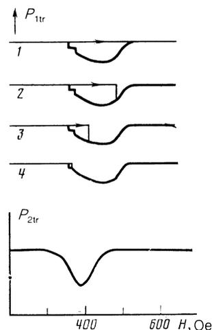
FIG. 3. The top part of the figure shows the microwave power transmitted by the resonator at  $\omega_{p1}/2\pi = 35.6$  GHz for various values of the AFMR pump power of frequency  $\omega_{p2}/2\pi = 17.52$  GHz. The curves are labeled 1-4 in the increasing order of the AFMR pump power. The bottom of the figure shows the absorption curve corresponding to the AFMR at  $\omega_{p2}$ ;  $\mathbf{h}_{p1} \parallel \mathbf{H}$ ,  $\mathbf{h}_{p2} \perp \mathbf{H}$ ,  $T = 1.2$  K.
