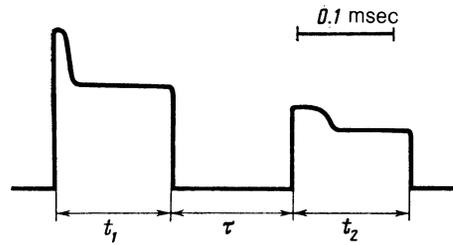
FIG. 5. Schematic representation of an oscillogram of the microwave signal transmitted by the resonator in the experiment with two pump waves applied at different times:  $t_1$  and  $t_2$  are the durations of the pump pulses at frequencies  $\omega_{p1}$  and  $\omega_{p2}$ .
