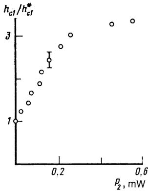
FIG. 4. Dependence of the ratio of the threshold field  $h_{c1}$  for the parametric excitation of magnons at  $\omega_{p1}/2\pi = 35.6$  GHz to the threshold field  $h_{c1}^*$ , measured in the presence of AFMR pumping at  $\omega_{p2}/2\pi = 17.52$  GHz, on the frequency  $\omega_{p2}$  of the pump power absorbed by the sample;  $H = 370$  Oe,  $T = 1.2$  K.
