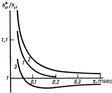
FIG. 6. Dependences of the ratio of the threshold field  $h_{c1}^*$  for the parametric excitation of magnons at  $\omega_{p2}/2\pi = 26.3$  GHz, measured in the presence of preliminary pumping at  $\omega_{p1}/2\pi = 35.6$  GHz, to the unperturbed value of  $h_{c1}$  on the time interval  $\tau$  between the pulses ( $T = 1.2$  K): 1)  $H = 180$  Oe; 2) 183 Oe; 3) 183.5 Oe.
