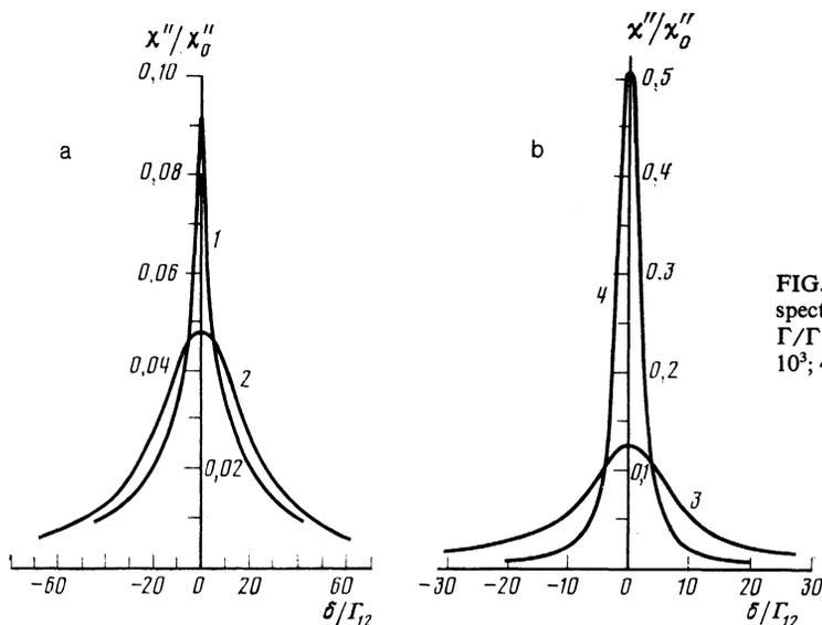
FIG. 6. Evolution of the absorption line profile due to variation of the spectral width of the noise field in the case of an exact resonance ( $\Delta = 0$ ,  $\Gamma/\Gamma_{12} = 3 \times 10^2$ ,  $\Omega_R^2/\Gamma\Gamma_{12} = 0.66 \times 10^2$ ); 1)  $\gamma/\Gamma_{12} = 10^{-2}$ ; 2)  $10^2$ ; 3)  $10^3$ ; 4)  $10^4$ .
