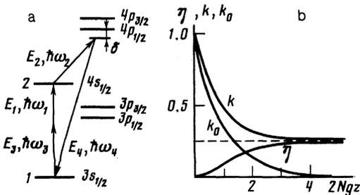
FIG. 1. (a) Schematic representation of the energy levels and of the interacting waves. (b) Dependences of the conversion efficiency  $\eta$  and of the transmission coefficient of the signal waves  $k$  and  $k_0$  on the length  $z$  of the nonlinear medium in the case when  $g_3 = g_4$ .
