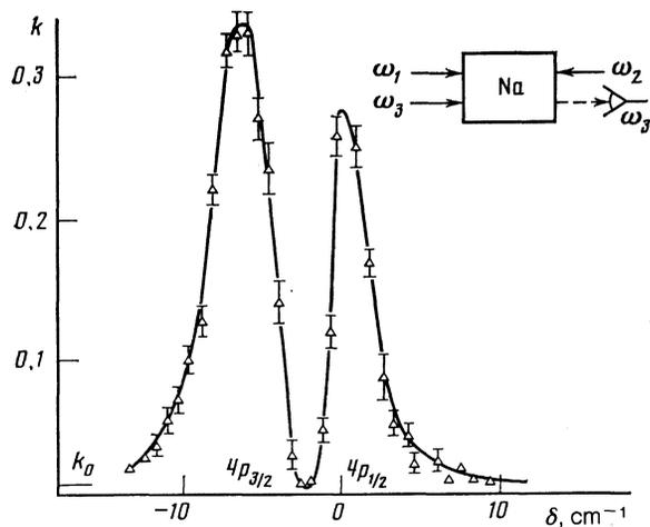
FIG. 3. Dependences of the transmission coefficient of the signal wave on the frequency of the second pump wave. The intensities of the pump waves were  $I_1 = 12 \text{ MW/cm}^2$  and  $I_2 = 100 \text{ kW/cm}^2$ . The sodium vapor concentration was  $7 \times 10^{15} \text{ cm}^{-3}$ .
