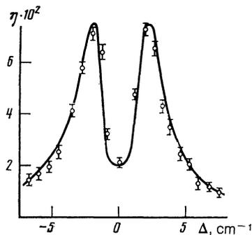
FIG. 7. Spectral dependence of the conversion efficiency Pump wave intensities  $I_1 = 5 \text{ MW/cm}^2$  and  $I_2 = 60 \text{ MW/cm}^2$ . The sodium vapor concentration was  $N = 4 \times 10^{16} \text{ cm}^{-3}$ .
