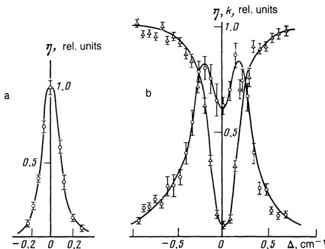
FIG. 6. Dependences of the conversion efficiency  $\eta$  (O) and of the signal radiation transmission coefficient  $k$  ( $\Delta$ ) on the detuning from a two-photon resonance. The intensities of the pump waves were  $I_1 = 40 \text{ MW/cm}^2$  and  $I_2 = 50 \text{ kW/cm}^2$ . The concentration of the sodium vapor was  $N = 10^{12} \text{ cm}^{-3}$  (a) and  $3.5 \times 10^{15} \text{ cm}^{-3}$  (b). The continuous curves are drawn by hand.
