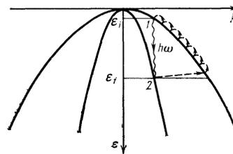
FIG. 1. Scheme of optical transitions and subsequent energy relaxation of heavy holes.
