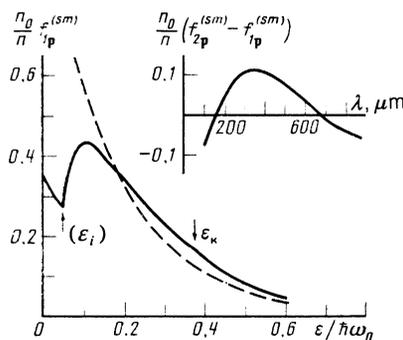
FIG. 2. Smooth part of heavy-hole distribution function vs the hole energy (referred to the optical-phonon energy  $\hbar\omega_0$ ), calculated from Eq. (29) for  $p$ -Ge,  $\lambda = 100 \mu\text{m}$ ,  $T = 77.4$  K, and  $Z = 5$ . The dashed curves show the equilibrium distribution ( $Z = 0$ ). The inset shows the dependence of  $f_{2p}^{(sm)} - f_{1p}^{(sm)}$  on the radiation wavelength  $\lambda$  corresponding to a vertical transition with momentum  $\mathbf{p}$ .
