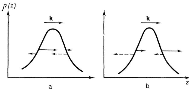
FIG. 2. Illustration of the stabilization (a) and spreading (b) of a drifting particle clump.
