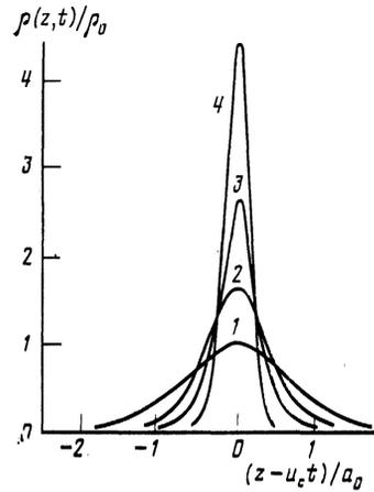
FIG. 5. Evolution of a single particle clump. The width  $a_0$  of the initial distribution is greater than  $D/\Delta u$  of the solitary wave.  $\alpha = 0.1$ ;  $u_c a_0/2D = 50$ ;  $t' = t\Delta u/a_0$ . Curve 1— $t' = 0$ ; 2— $t' = 1$ ; 3— $t' = 2$ ; 4— $t' > 10$ .
