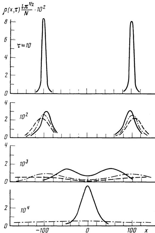
FIG. 7. Evolution of two particle clumps:  $L\Delta u/D \gg 1$ ,  $\tau = u_c^2 t/D$ ,  $L/l = 200$ ,  $l = D/u_c$ ,  $\alpha = \Delta u/2u_c$ . Solid curve— $\alpha = 0.1$ , dot-dash curve  $\alpha = 0$ , dashed curve— $\alpha = -0.1$ .
