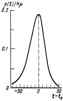
FIG. 8. Shape of solitary wave for  $\partial u(z,t)/\partial N(z,t) = 0$ ;  $\alpha = 0.1$ .
