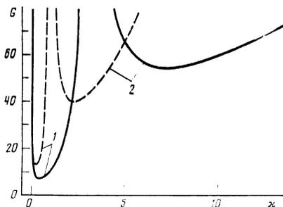
FIG. 9. Width of solitary wave as a function of radiation intensity. Curve 1— $\Omega \Delta \nu < 0$ , 2— $\Omega \Delta \nu > 0$ ; solid curve— $\beta = 0.1$ ; broken curve  $\beta = 1$ .
