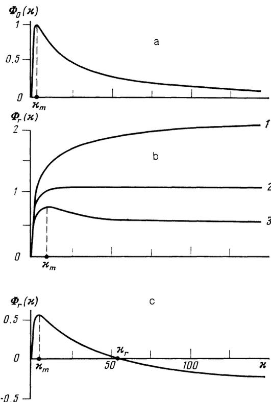
FIG. 1. Drift velocity as a function of radiation intensity: (a) LID effect,  $\beta = 0.1$ ; (b) radiation pressure effect for  $\Delta\nu/2\Gamma_1 < 1$ . Curve 1— $\Delta\nu/\nu = -0.1$ ,  $\Delta\nu/2\Gamma_1 = -1$ ,  $\beta = 1/21$ , 2— $\Delta\nu = 0$ , 3— $\Delta\nu/\nu = 0.1$ ,  $\Delta\nu/2\Gamma_1 = 0.5$ ,  $\beta = 1/11$ ; (c) radiation pressure effect for  $\Delta\nu/2\Gamma_1 > 1$ ,  $\Delta\nu/\nu = 0.1$ ,  $\Delta\nu/2\Gamma_1 = 1.5$ ,  $\beta = 1/31$ .
