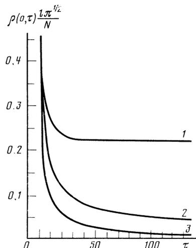
FIG. 3. Particle clump amplitude as a function of time:  $\tau = u_c^2 t/D$ . Curve 1— $\alpha = 0.5$ ; 2— $\alpha = 0$ ; 3— $\alpha = -0.5$ .
