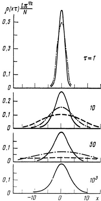
FIG. 4. Evolution of a single particle clump. The width  $a_0$  of the initial distribution is less than the width  $D/\Delta u$  of the solitary wave: solid curve— $\alpha = 0.5$ ; dot-dash curve— $\alpha = 0$ ; dashed curve— $\alpha = -0.5$ .
