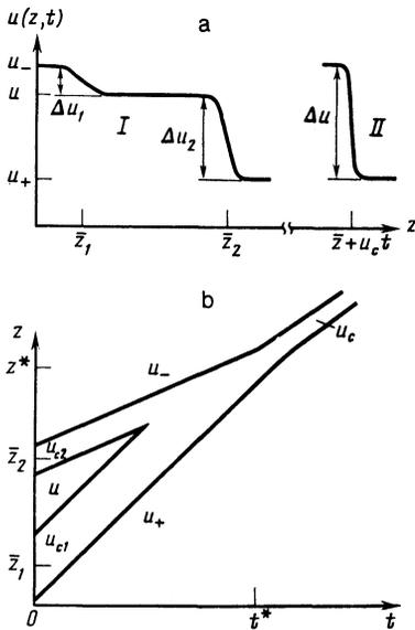
FIG. 6. (a) Drift velocity  $u(z, t)$  as a function of  $z$  for (3.6);  $L \gg a_0$ ,  $\sigma > 0$ . (I)  $t = 0$ ; (II)  $t \gg L/\Delta u$ . (b) Analogy with the collision between two shock waves.
