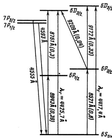
FIG. 1. Energy-level scheme of the cesium atom.
