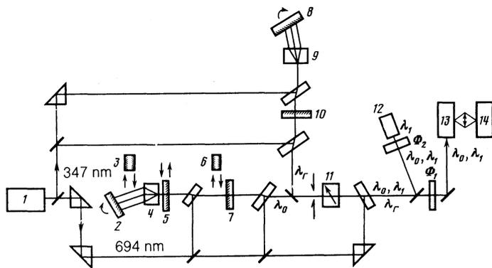
FIG. 2. Block diagram of the apparatus: 1—source of radiation with  $\lambda = 694$  and  $347$  nm; 2, 8—diffraction grating; 3, 6—Fabry-Perot interferometers; 4, 9—prism beam expanders; 5—mirror with  $R = 100\%$ ; 7, 10—exit mirrors; 11— $\text{LiIO}_3$  crystal mixer; 12, 14—photodetectors; 13—cell containing cesium vapor.
