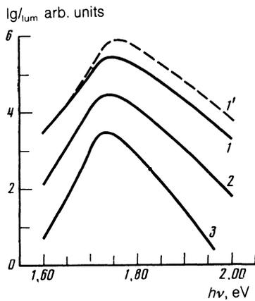
FIG. 1. Luminescence spectra for a CdSe single crystal (E1c) with  $h\nu_0 = 2.15$  eV and pump intensity  $I = I_0 = 6 \cdot 10^{24}$  photons/(cm<sup>2</sup>·s) (1),  $I = 0.24I_0$  (2),  $I = 0.03I_0$  (3); 1') spectrum 1 corrected for reabsorption. The intensity scale for each spectrum is shifted arbitrarily.
