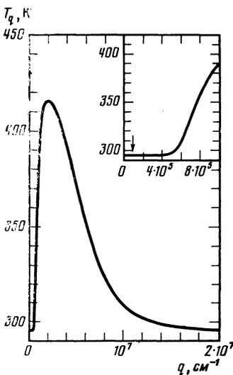
FIG. 4. Calculated spectrum for the excess  $LO$  phonons,  $h\nu_0 = 2.15$  eV,  $I = I_0$ ,  $T_e = 450$  K. In the insert showing the small- $q$  region, the arrow indicates the maximum wave number for a phonon capable of participating in first-order Raman light scattering for a probing light beam with  $h\nu_0 = 2.15$  eV.
