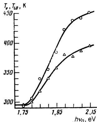
FIG. 3. Experimental dependence of the effective excess carrier (O) and LO-phonon ( $\Delta$ ) temperature as functions of the laser photon energy for CdSe,  $I = I_0$ .
