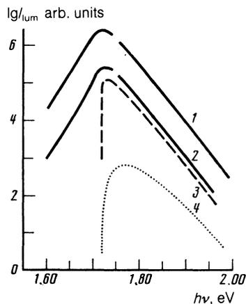
FIG. 2a,b. As in Fig. 1, but for  $h\nu_0 = 1.75$  eV:  $I = I_0$  (1),  $I = 0.03I_0$  (2); (3, 4) show the theoretical luminescence spectra for an electron-hole plasma with  $T_e = 295$  K and  $\bar{E}_g = 1.72$  eV and the quasimomentum selection rules for interband transitions are (3) and are not obeyed (4).
