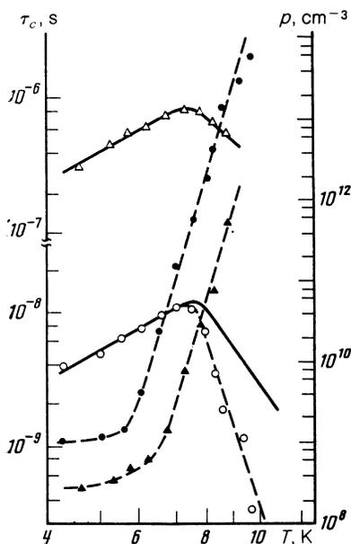
FIG. 4. Plots of  $\tau_c(T)$  and  $p(T)$  for  $p$ -Ge. Sample No. 8:  $\Delta$ — $\tau_c$ ,  $\blacktriangle$ — $p$ ; sample No. 12:  $\circ$ — $\tau_c$ ,  $\bullet$ — $p$ .
