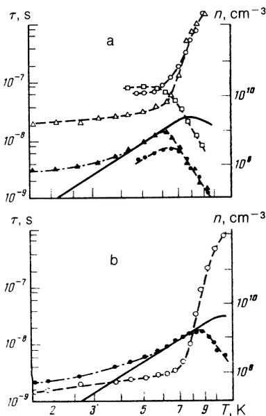
FIG. 1. Plots of  $\tau_c(T)$ ,  $\tau_p(T)$  and  $n(T)$  for *n*-Ge. a) Sample No. 4:  $\blacktriangle$ — $\tau_c$ ,  $\square$ — $\tau_p$ ,  $\triangle$ — $n$  and  $I < I_k$ ,  $\bullet$ — $\tau_c$ ,  $\circ$ — $n$  and  $I > I_k$ . b) Sample No. 5:  $\bullet$ — $\tau_c$ ,  $\circ$ — $n$  and  $I < I_k$ .
