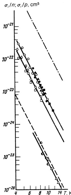
FIG. 7. Temperature dependences of  $\sigma_i/n$ ,  $\sigma_i/p$ . The results correspond to  $n$ -Ge samples:  $\blacktriangle$ —No. 3,  $\circ$ —No. 4,  $\blacksquare$ —No. 5;  $p$ -Ge without compression:  $\triangle$ —No. 11,  $\bullet$ —No. 12;  $p$ -Ge under strong compression:  $\diamond$ —No. 8,  $\square$ —No. 9. The plots calculated from (1) and (2) are dash-dot and dashed, respectively.
