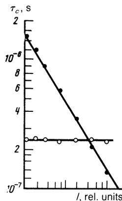
FIG. 6. Plots of  $\tau_c(I)$  for sample 8 under strong uniaxial compression (●) and without compression (○),  $T = 4.2 \text{ K}$ .
