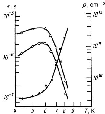
FIG. 5. Plots of  $\tau_c(T)$  (○),  $\tau_p(T)$  (△),  $p(T)$  (●) for sample No. 8 ( $p$ -Ge) under strong uniaxial compression.
