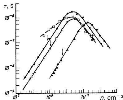
FIG. 2. Plots of  $\tau_c(n)$  for samples No. 5— $\bullet$ , No. 6— $\blacktriangle$ , No. 7— $\circ$  and of  $\tau_p(n)$  for sample No. 7— $\square$  at *n*-Ge and  $T = 4.2 \text{ K}$ ,  $I < I_k$ . The arrows mark the changes of *n* corresponding to the start of the vertical sections of the current-voltage characteristics of the samples at breakdown.
