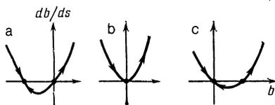
FIG. 2. Phase portrait of the renormalization-group equation (20) for different dimensionalities of space: a)  $d < 2$ ; b)  $d = 2$ ; c)  $d > 2$ .
