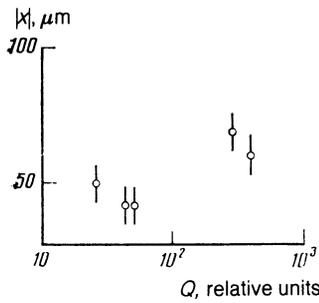
FIG. 2. Distance at which a periodic structure's amplitude decreases by a factor of two as a function of radiation intensity.
