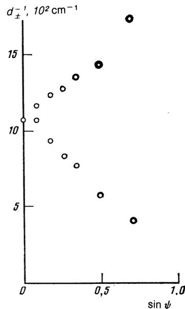
FIG. 4. Dependence of the structure period  $d_{\perp}$  on the incidence angle  $\psi$  for the case when the vector  $\mathbf{E}$  in the incident lightwave is parallel to the incidence plane.
