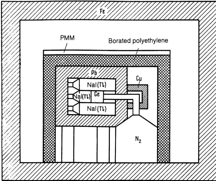
FIG. 1. Apparatus used in the search for sodium-24 gammas.
