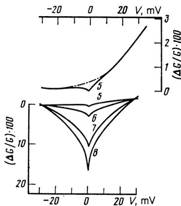
FIG. 6. Dependences  $\Delta G(V)/G$  obtained for tunnel contacts with three-dimensional disordered electrodes at  $T = 0.4 \text{ K}$  in  $H = 35 \text{ kOe}$ . The numbers of the samples are indicated alongside the curves. The dash-dot curve is a parabolic dependence  $\Delta G(V)/G$  observed for pure samples and associated with barrier effects.
