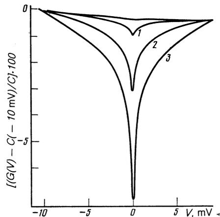
FIG. 2. Dependences  $\Delta G(V)/G$  obtained at  $T = 0.4$  K in  $H = 35$  kOe for tunnel contacts with two-dimensional disordered electrodes. The numbers of the samples are given alongside each curve. The highest curve was obtained for a tunnel contact formed by films of thickness  $l > 1000$  Å.
