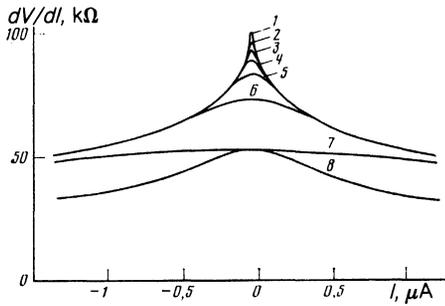
FIG. 8. Dependences  $(dV/dI)(I)$  for tunnel contacts in which the disordered electrode was film No. 8, obtained at the following temperatures: 1) 0.4 K; 2) 4.2 K; 3) 10 K; 4) 20 K; 5) 40 K; 6) 90 K; 7), 8) 300 K. Curve 8 is plotted on a current scale different from the rest of the figure: one division represents  $2\mu A$ .
