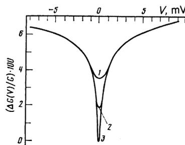
FIG. 4. Dependences  $\Delta G(V)/G$  obtained for tunnel contacts in which the disordered electrode was film No. 3, obtained in  $H = 35$  kOe at the following temperatures: 1) 4.2 K; 2) 1.3 K; 3) 0.4 K.
