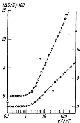
FIG. 3. Dependences of  $\Delta G/G$  on  $eV/kT$  for tunnel contacts in which the disordered electrodes were films Nos. 3 ( $\circ$  and  $\blacksquare$ ) and 4 ( $\bullet$  and  $\square$ ), obtained in  $H = 35$  kOe at various temperatures:  $\circ$ ) 0.4 K;  $\square$ ) 0.6 K;  $\bullet$ ,  $\blacksquare$ ) 4.2 K. The dashed curves are the theoretical dependences represented by Eq. (6).
