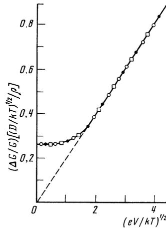
FIG. 7. Normalized dependences of  $\Delta G/G$  on  $eV/kT$  for tunnel contacts in which the disordered electrode was film No. 6, obtained in  $H = 35 \text{ kOe}$  at  $T = 0.4 \text{ K}$  (●),  $1.3 \text{ K}$  (○), and  $4.2 \text{ K}$  (□). The continuous curve is the theoretical dependence represented by Eq. (7).
