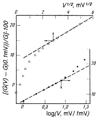
FIG. 5. Dependences of  $\Delta G(V)/G$  on  $V^{1/2}$  (O) and on  $\ln(V, \text{mV}/1 \text{mV})$  (●), obtained at  $T = 0.4 \text{ K}$  in  $H = 35 \text{ kOe}$  for tunnel contacts in which the disordered electrode was film No. 4.
