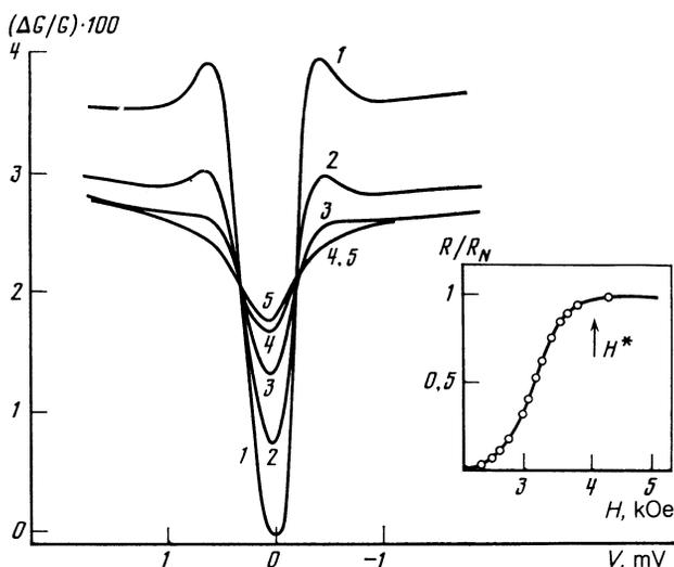
FIG. 1. Dependences  $\Delta G(V)/G$  obtained at  $T = 0.4$  K for tunnel contacts in which the disordered electrode was film No. 1. The intensities of the magnetic field oriented at right-angles to the film plane were (kOe): 1) 0.9; 2) 3.5; 3) 9.0; 4) 17.5; 5) 35. The inset shows the dependence  $R(H)/R_N$  for film No. 1 at  $T = 0.4$  K.
