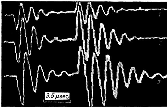
FIG. 2. Free vibrations of a Bloch line initiated by pulses of a magnetic field  $H_x$  of different amplitudes: 1)  $H_0 = 6.5$  mOe; 2) 9.7; 3) 13.0;  $\tau = 7$   $\mu\text{sec}$ ,  $T = 200$   $\mu\text{sec}$ .
