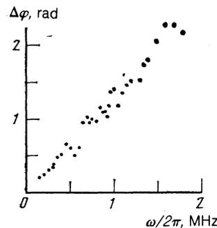
FIG. 4. Frequency dependence of the difference between the phases of harmonic vibrations of a domain wall determined near a current-carrying conductor and at a distance of 3 mm from it.
