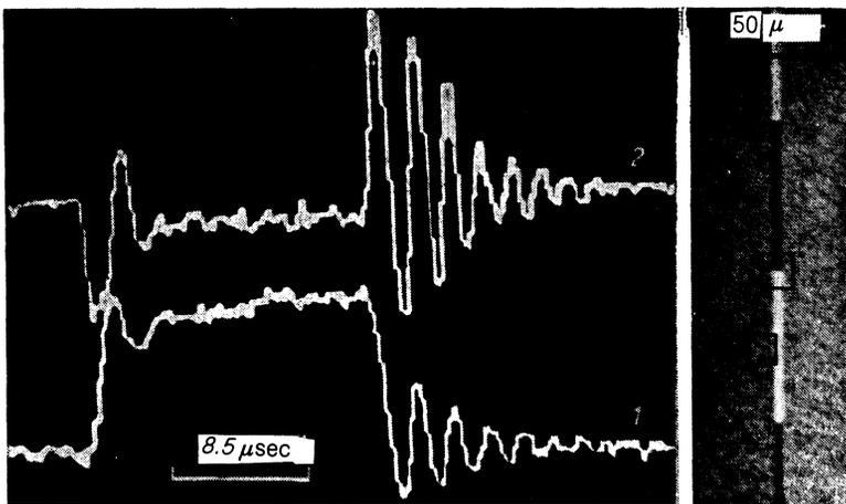
FIG. 1. Free damped vibrations of a domain wall (curve 1) and of a Bloch line (curve 2) induced by a magnetic field pulse  $H_x$  of amplitude 22.4 mOe, duration  $\tau = 15 \mu\text{sec}$ , and repetition period  $T = 200 \mu\text{sec}$  (the signals were displayed on the screen of a visual display unit after storage in a computer memory). The photograph on the right shows a domain wall with identification of the regions subjected to photometric analysis in recording curves 1 and 2.
