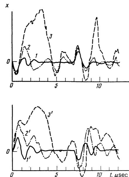
FIG. 6. Free vibrations of neighboring Bloch lines under the action of magnetic field pulses of the following amplitudes  $H_0$  (mOe): 1) 15; 2) 25; 3) 30;  $\tau = 7$   $\mu$ sec,  $\nu = 200$  Hz.
