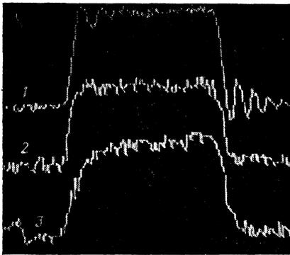
FIG. 8. Motion of a domain wall (containing Bloch lines) under the action of magnetic field pulses of different amplitudes  $H_0$  (mOe): 1) 28; 2) 50; 3) 100;  $\tau = 15 \mu\text{sec}$ ,  $T = 200 \mu\text{sec}$ .
