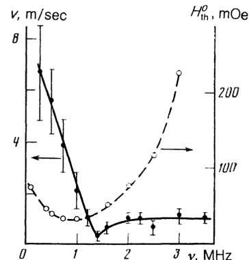
FIG. 11. Frequency dependences of the threshold amplitude ( $H_{th}^0$ ) of a sinusoidal field above which excitations of soliton waves begin and the velocities ( $v$ ) of their motion, measured for  $H_x^0 = H_{th}^0$ ;  $H_z = 15$  Oe.
