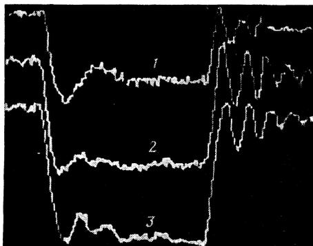
FIG. 9. Motion of a one-dimensional domain wall under the action of magnetic field pulses of different amplitudes  $H_0$  (mOe): 1) 20.2; 2) 22.4; 3) 24.6;  $\tau = 4 \mu\text{sec}$ ,  $T = 200 \mu\text{sec}$ ;  $H_z = 18$  Oe.
