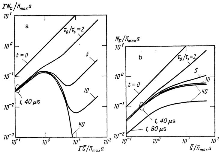
FIG. 2. Total number of nonequilibrium carriers in the sample vs the pump level at various instants of time  $t$  following the excitation pulse, for several values of the ratio  $\tau_0/\tau_s$ . a) Phonon wind emitted by hot spot. Calculation from Eq. (7a). b) Phonon wind emitted by the EHD themselves. Calculation from Eq. (7b).
