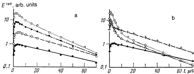
FIG. 3. EHD luminescence kinetics in Ge samples of thickness  $a = 0.1$  mm at various pump levels  $J/J_{\max} = 1.0$  (○), 0.40 (●), 0.12 (□), 0.03 (■), 0.59 (△), 0.04 (▲), 0.41 (+) ( $J_{\max} = 120$  erg). The samples were etched for 1.5 min (a) and 1 min (b).
