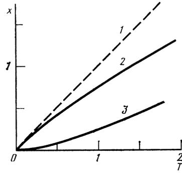
FIG. 3. Evolution of the reduced vector potential and of the axial electron current with time in the stage of the formation of the REB. We have put:  $I_* = mc^3/2|e|\epsilon$ ; 1:  $x^0(T)$ , 2:  $x(T)$ , 3:  $I_n/I_*$ .
