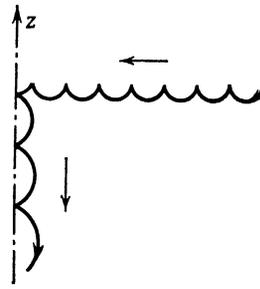
FIG. 2. Qualitative picture of the electron drift in the near-axial region of the constriction. The arrows indicate the direction of the drift.
