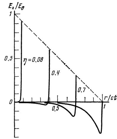
FIG. 4. Profile of the fast electromagnetic rarefaction wave in successive instants of time. The parameter of the curves is  $\eta = ct/R_*$ ;  $\epsilon = 0.2$ .
