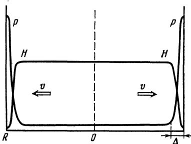
FIG. 1. Profiles of the pressure and the magnetic field during the compression of the plasma by the liner.
