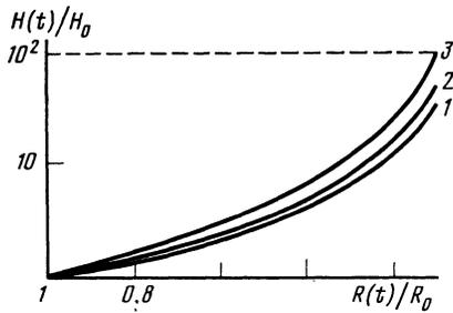
FIG. 3. Profiles of the magnetic field in the plasma for various values of the effective magnetic Reynolds number  $R_{\text{eff}}^{(0)}$ : 1—10; 2—30; 3— $\infty$ .
