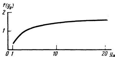
FIG. 5. The function  $f(y_0)$ , describing at  $y^* \ll 1$  the energy flux into the plasma [see Eq. (2.14)]. At  $y_0 \gtrsim 10$ , it is seen that the quantity  $Q$  is practically independent of  $y_0$  and  $\max f(y_0) = 1.6$ .
