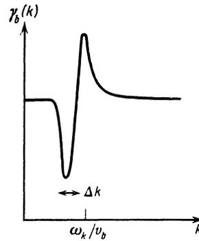
FIG. 2. The dependence of  $\gamma_b$  on the absolute value of the wave vector for a fixed value of  $y$ . The distribution function is chosen to have the form  $f_0 \propto \exp[-(v_{\perp} - v_b)^2/\Delta v^2]$ , where  $v_b = 10v_{Ti}$  and  $\Delta v = 0.1v_b$ .
