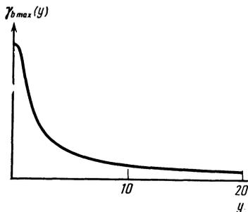
FIG. 1. The dependence of the maximum value  $\gamma_{b \max}$  of the growth rate of the beam instability on the parameter  $y = (M/m)^{1/2} \cos \theta$ .
