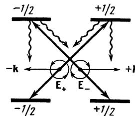
FIG. 1. Interaction scheme of an atom at the transition  $1/2 \rightarrow 1/2$  with field (1) in a cycle of the optical pump. The heavy lines with the two arrows correspond to the counterpropagating  $\sigma_\pm$  components of the wave. The wavy lines represent spontaneous decay.
