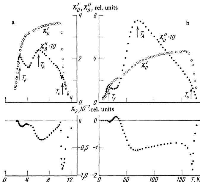
FIG. 3. Temperature dependences of the real part  $\chi'_0$  and imaginary part  $\chi''_0$  of the dynamic magnetic susceptibility, and nonlinear susceptibility  $\chi_2$ , of the alloys  $(\text{Pd}_{99.65}\text{Fe}_{0.35})_{95.0}\text{Mn}_{5.0}$  (a) and  $\text{Au}_{81}\text{F}_{19}$  (b). The measurement field has frequency 60 Hz and intensity 1 Oe (a) and 3 Oe (b).
