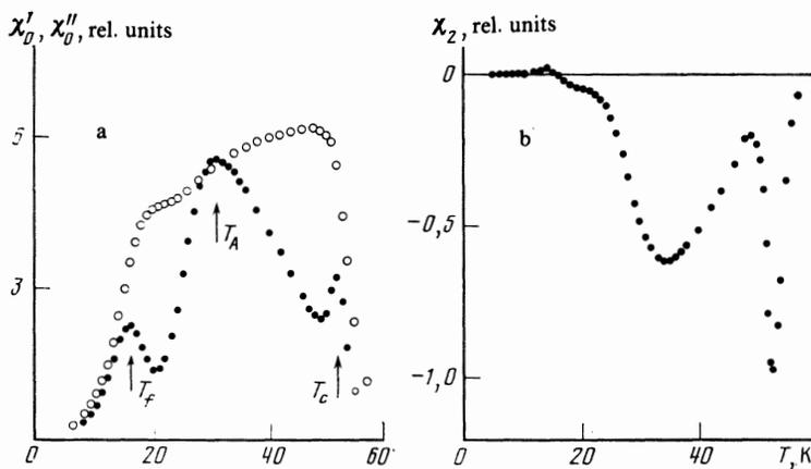
FIG. 1. Temperature dependences of a) the real part  $\chi'_0$  (the light circles) and imaginary part  $\chi''_0$  (the dark circles) of the dynamic magnetic susceptibility, and b) the nonlinear susceptibility  $\chi_2$  of the alloy  $\text{Fe}_{54}\text{Ni}_{26}\text{Cr}_{20}$ . The measurement field has intensity 1 Oe and frequency 60 Hz.
