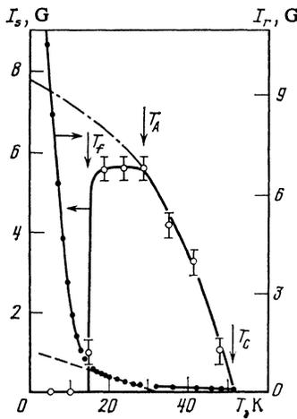
FIG. 2. Temperature dependences of the spontaneous magnetization  $I_s$  and residual magnetization  $I_r$  of the alloy  $\text{Fe}_{5.4}\text{Ni}_{26}\text{Cr}_{20}$ .
