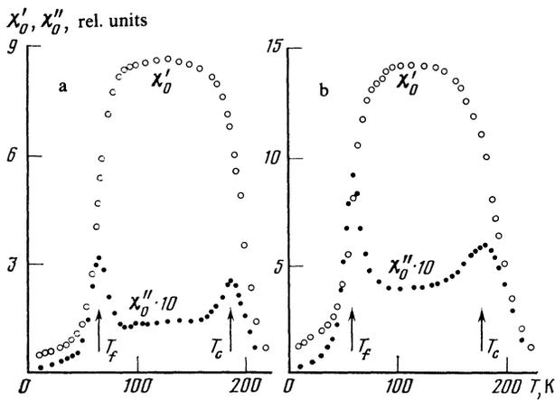
Fig. 4. Temperature dependences of the real part  $\chi'_0$  and imaginary part  $\chi''_0$  of the dynamic magnetic susceptibility of the alloys  $\text{Fe}_{52.5}\text{Ni}_{32.5}\text{Mn}_{15.0}$  (a) and  $\text{Ni}_{77.9}\text{Mn}_{22.1}$  (b). The measurement field has intensity 1 Oe and frequency 36 Hz.
