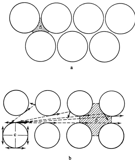
FIG. 2. A periodic Lorentz gas: a) with a bounded free path; b) with an unbounded free path; c) singular trajectories;  $B$  is a unit cell of the configuration.
