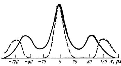
FIG. 2. Autocorrelation functions of radiation at the pump frequency during SRS in a fiber for different pump levels: equal to  $P_p$ —broken curve, greater than  $P_p$ —solid curve.
