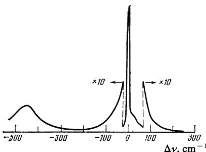
FIG. 1. Spectrum at exit from an optical fiber pumped by laser pulses with  $\lambda_p = 1.064 \mu\text{m}$  and  $\tau_p = 60 \text{ ps}$ .
