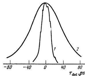
FIG. 3. Autocorrelation function at the frequency of the first Stokes component of SRS (curve 1) and of the pump at entry to the fiber (curve 2).
