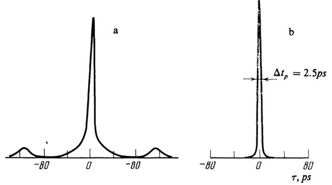
FIG. 4. Autocorrelation functions of radiation leaving an optical fiber in the anti-Stokes region relative to the pump: a— $\Delta\nu = \nu_a - \nu_p = 36 \text{ cm}^{-1}$ , b— $104 \text{ cm}^{-1}$ .
