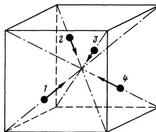
FIG. 1. Magnetic structure of  $\text{UO}_2$ . The ion magnetic moments are parallel to the body diagonals of the cube.
