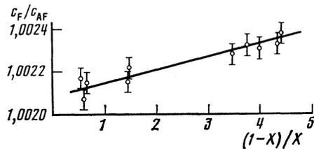
FIG. 5. The dependence of  $c_F/c_{AF}$  on  $(1-X)/X$  at 88.3 K.
