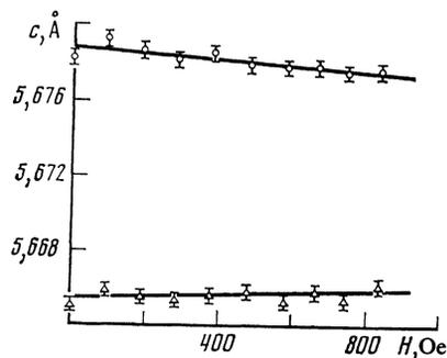
FIG. 2. The field dependence of the parameter  $c$  of dysprosium at  $88.3$  K, ○ F phase, △ AF phase.
