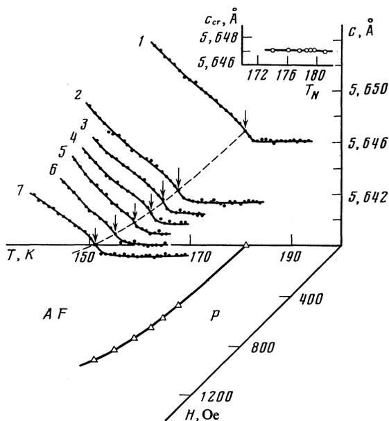
FIG. 3. The  $c$ - $H$ - $T$  diagram of Dy near  $T_N$ : 1)  $H = 0$ ; 2) 480 Oe; 3) 580 Oe; 4) 665 Oe; 5) 745 Oe; 6) 835 Oe; 7) 920 Oe. The inset shows the dependence of  $c_{cr}$  (at the P-AF transition point) on the temperature of the phase transition.
