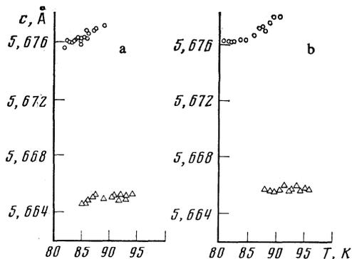
FIG. 1. The temperature dependence of the parameter  $c$  in the neighborhood of the temperature  $\Theta$  in fields  $H = 0$  (a) and  $H = 835$  Oe (b); ○ F phase, △ AF phase.
