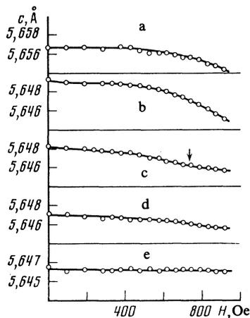
FIG. 4. The  $c(H)$  isotherms of dysprosium near  $T_N$ : a)  $T = 148.3$  K; b) 172 K; c) 178 K; d) 180.5 K; e) 184.2 K.
