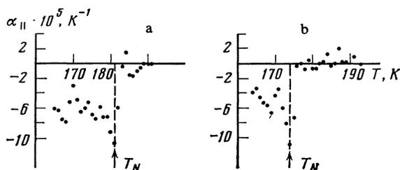
FIG. 6. The temperature dependences of the linear expansion coefficient  $\alpha_{\parallel}$  of dysprosium near  $T_N$  for  $H = 0$  (a) and  $H = 920$  Oe (b).
