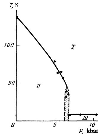
FIG. 3. the  $T$ - $P$  phase diagram of (BEDT-TTF) $_2$ I $_3$ . The temperatures of the phase transitions were determined for each pressure from the point of intersection of the linearly extrapolated sections of the  $\log R(T)$  curves (marked by arrows in Fig. 1).
