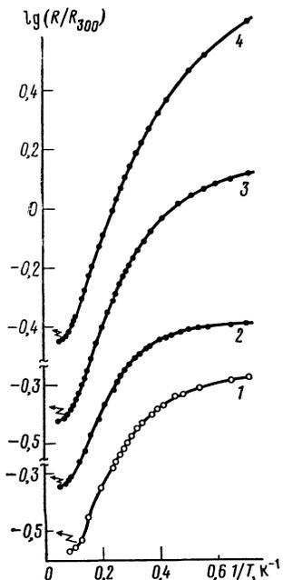
FIG. 2. The dependence of  $\log(R/R_{300})$  on  $1/T$  for specimens II (curve 1) and I (curves 2, 3, 4) at: 1) 9.1 kbar; 2) 9.3 kbar; 3) 11.1 kbar; 4) 13.9 kbar.
