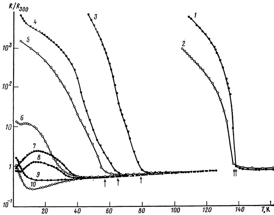
FIG. 1. The temperature dependences of the resistance of specimens I (●) and II (○) of  $\alpha$ -(BEDT-TTF) $_2$ I $_3$  at pressures of 1), 2) 1 kbar; 3) 6.3 kbar; 4) 7.5 kbar; 5) 7.9 kbar; 6) 8.5 kbar; 7) 8.3 kbar; 8) 9.0 kbar; 9) 9.3 kbar; 10) 9.1 kbar. All values of pressure refer to room temperature.
